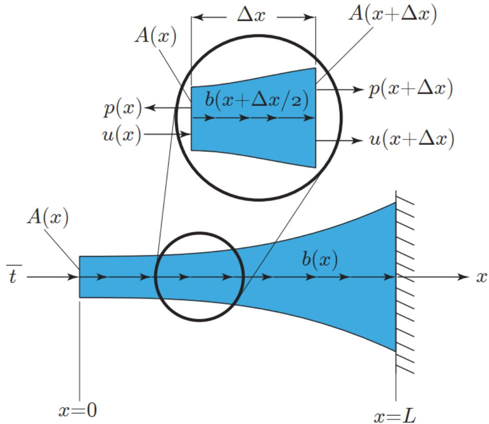
Figure 2.1: A one-dimensional stress analysis (elasticity) problem
