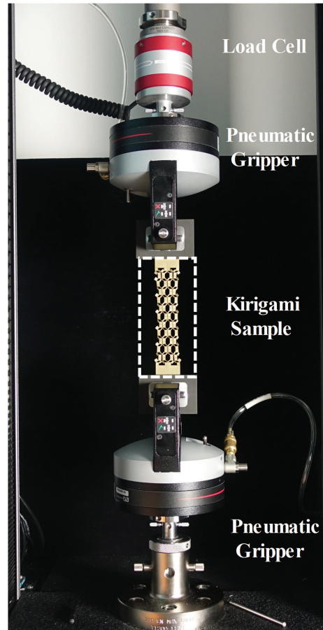
Figure S3: Experimental setup. Our kirigami samples are stretched uniaxially using an Instron tensile machine.
